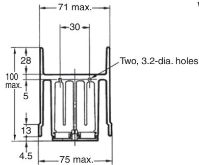
**Y92B-N150 Heat Sink (for the G3NB-225B-1, G3NB-240B-1)**
