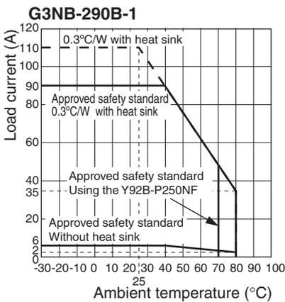
**Note:** Ventilated of FAN; 0.22 m<sup>3</sup>/min
