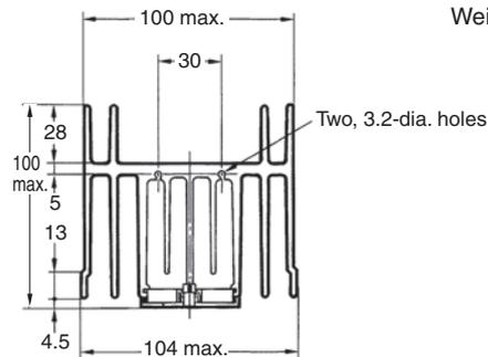
**Y92B-P250NF Heat Sink (for the G3NB-275B-1, G3NB-290B-1)**
