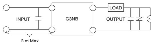
Recommended Capacitor (Film Capacitor) Load: 0.1 μF, 275 VAC
