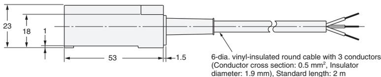
6-dia. vinyl-insulated round cable with 3 conductors (Conductor cross section: 0.5 mm<sup>2</sup>, Insulator diameter: 1.9 mm), Standard length: 2 m
