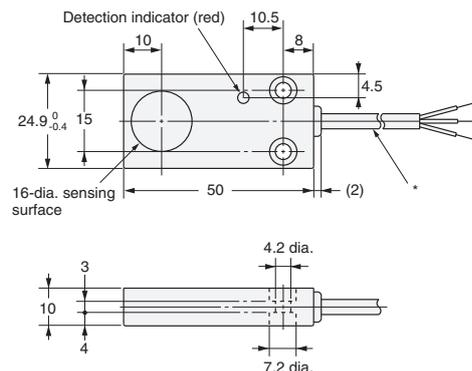
\* 4-dia. vinyl-insulated round cable with 3 conductors (Conductor cross section: 0.2 mm<sup>2</sup>, Insulator diameter: 1.2 mm), Standard length: 2 m
