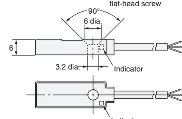
\* 2.9-dia. vinyl-insulated round cable with 3 conductors (Conductor cross section: 0.14 mm<sup>2</sup>, Insulator diameter: 0.9 mm), Standard length: 2 m
