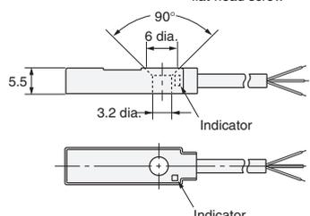
\* 2.9-dia. vinyl-insulated round cable with 3 conductors (Conductor cross section: 0.14 mm<sup>2</sup>, Insulator diameter: 0.9 mm), Standard length: 2 m
