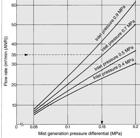
EX: How to obtain the mist generating pressure differential if the flow rate obtained in 1. above is 35 m³/min (ANR) and the line pressure (inlet pressure  $P_1$ ) is 0.7 MPa:
