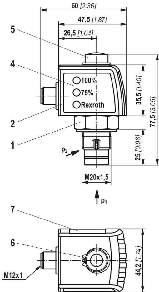
Pressure differential indicator with mounted switching element EN-175301-803
