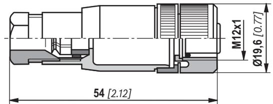
Mating connector suitable for K24-3m 4-pole, M12 x 1 with potted-in PVC cable, 3 m long.
